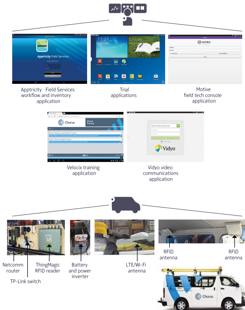
Figure 2. Technician’s tablet screen shots and the platform physical implementation
